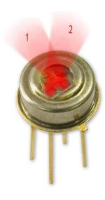
The thermopile sensor inside the MRAKOMĚR is covered by a small and thin HDPE cupola which protects the senor itself against atmospheric events. The HDPE material has good transparency in IR and it is hydrophobic. In case of big humidity there is 2W heating resistor inside the MRAKOMĚR. This heating is necessary against water vapor condensation on the sensor. This heating can melt accidental ice or snow as well.
