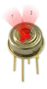
The thermopile sensor inside the MRAKOMĚR is covered by a small and thin HDPE cupola which protects the senor itself against atmospheric events. The HDPE material has good transparency in IR and it is hydrophobic. In case of big humidity there is 2W heating resistor inside the MRAKOMĚR. This heating is necessary against water vapor condensation on the sensor. This heating can melt accidental ice or snow as well.
