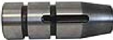
**Load pin** - load pin cells are designed to be installed in the axis of a sheave, shackle etc. through which force is applied. Most common load pins will measure force in one direction only. The direction of force is often marked with an arrow at one end of the pin or instructions for alignment may be given in the load cell certificate. If the load is off axis, the output will be reduced. At 90 degrees off axis the output will not change with a change in load.
