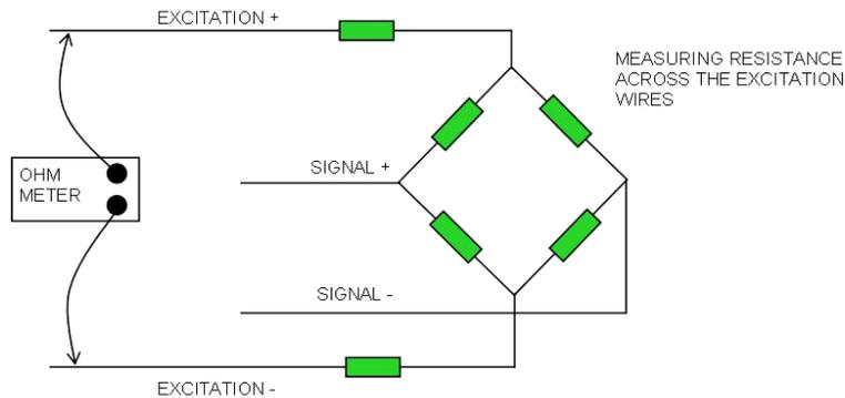
To test the cell obtain a meter capable of measuring Ohms, measure across each pair of wires in turn and record the results (space provided in the table which follows). The load cell must be completely disconnected from the monitor and at no load when these tests are made.
