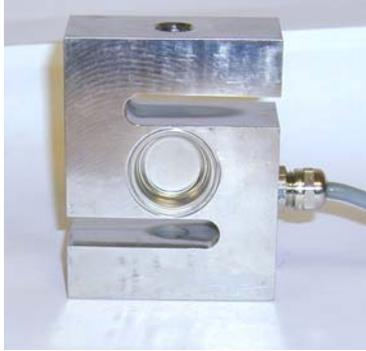
**S type** - the S type load cell can be used in tension and compression. The signal voltage output will reverse in polarity when the force changes from tension to compression i.e. the display value may change from. **Tension** load cells and **Load links** are designed to operate under tension only.
