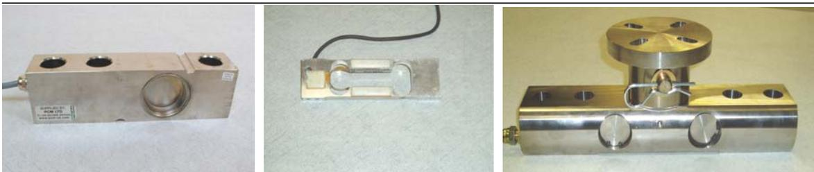
**Shear beam** - the shear beam load cell is fixed rigidly at one end with the force being applied to the other end. These can be used singly or in groups e.g. a platform scale using one cell in each corner.
