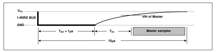
Figure 16. Recommended Master Read 1 Timing
