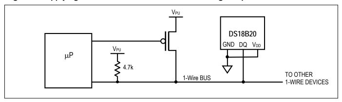
Figure 5. Powering the DS18B20 with an External Supply
