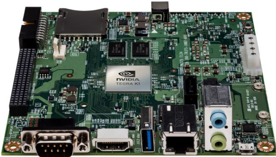
Figure 4.2. The NVIDIA Jetson TK1 Development Kit [27].
