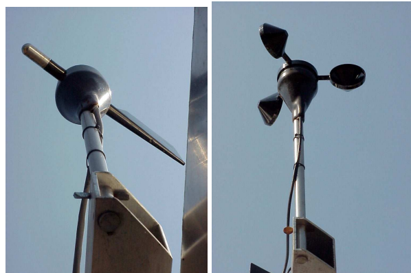
Figure 18. A lock screw under the wind vane direction boot (left), permits alignment with north. A co-located anemometer (right) measures wind speed.
