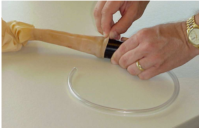
Figure 32. Inserting the check valve holder into the balloon neck.
