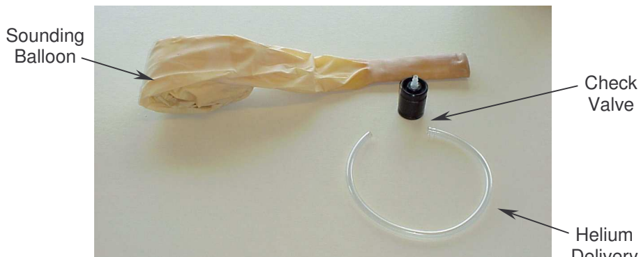
Figure 30. Expendable balloon components include the sounding balloon, gas check valve, and \approx 12 " (25 cm) piece of \frac{1}{4} " (6.4 mm) ID PVC tubing.
