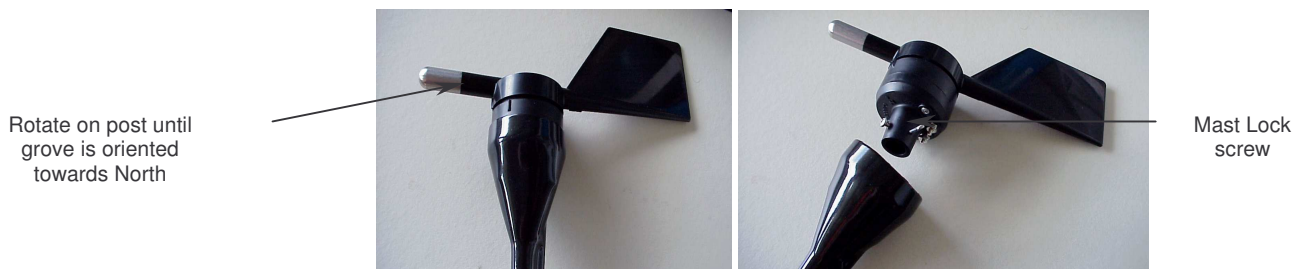
Figure 19. Aligning the wind direction sensor to geographical north.
