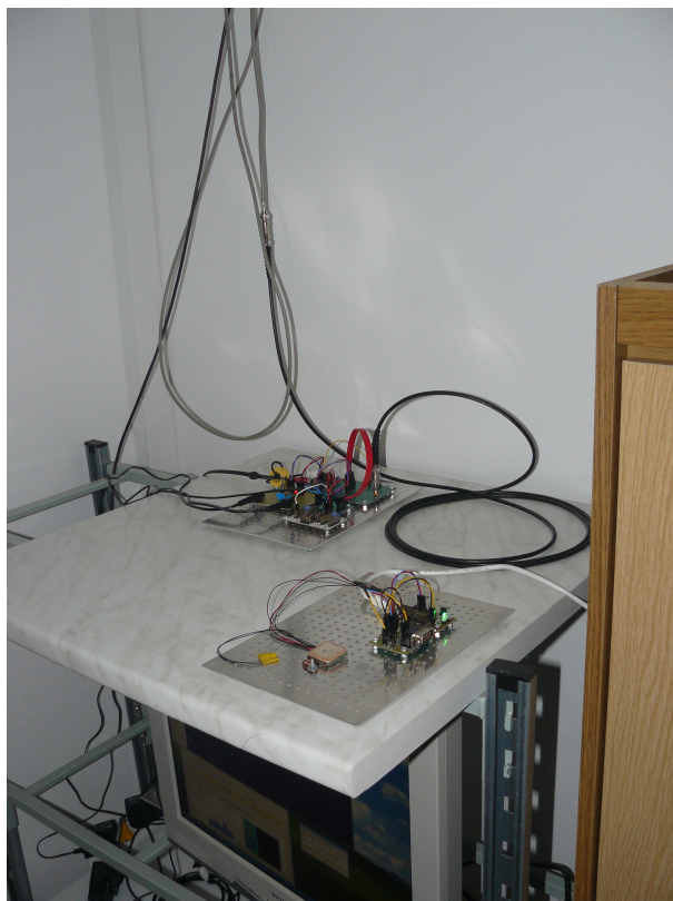
Obrázek 2: Example of meteor detector receiver setup
