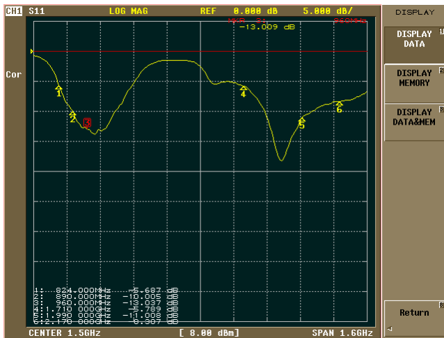
Figure 51: |S_{11}| sample measurement of a penta-band antenna that covers in a small form factor the 4 GSM bands (850 MHz, 900 MHz, 1800 MHz and 1900 MHz) and the UMTS Band I
