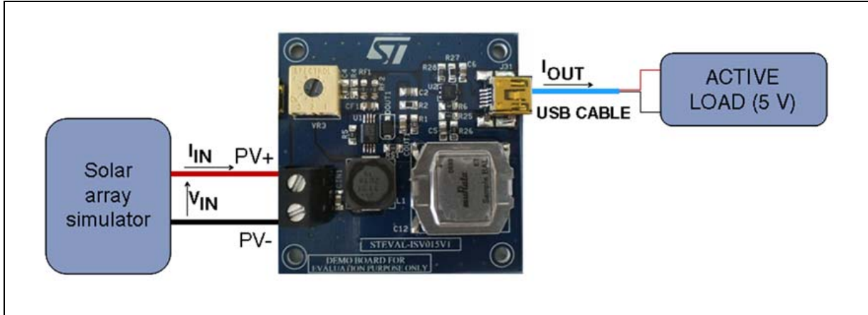
Figure 7. Supply and load connections
