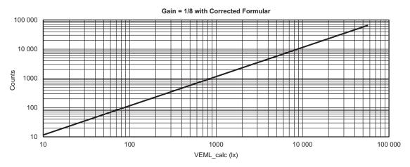
Fig. 14 - Linearity (counts vs. lux) for Gain 1/8 with Applied Correction Formula
