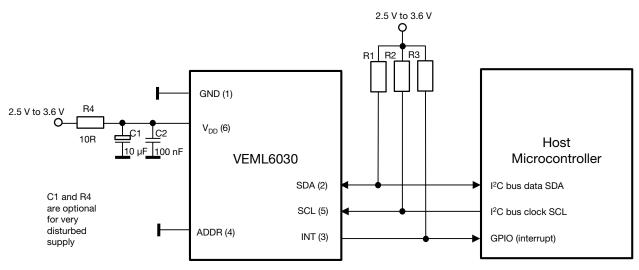
Fig. 2 - VEML6030 Application Circuit
