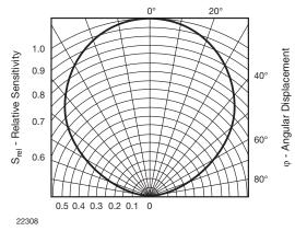
Fig. 22 - Relative Radiant Sensitivity vs. Angular Displacement
