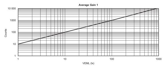
Fig. 8 - Linearity for Gain 1: Digital Counts vs. Lux\_VEML
