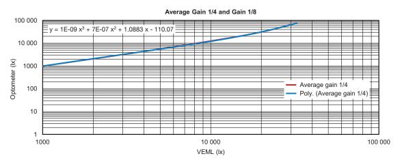
Fig. 12 - Correction Formula for Gain 1/4 and Gain 1/8 for Higher Light Levels Higher than 1000 lx
