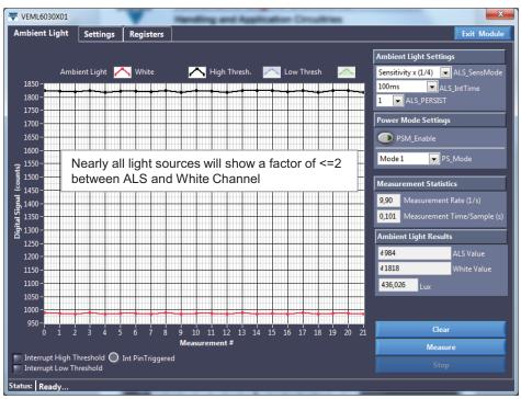
Fig. 19 - White Channel and ALS Channel for Fluorescent and Daylight Spectra
