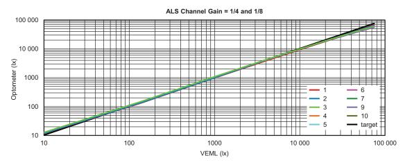
Fig. 13 - Linearity for Gain 1/4 and Gain 1/8 with Applied Correction Formula
