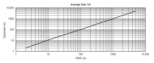
Fig. 9 - Linearity for Gain 1/4: Lux\_Optometer vs. Lux\_VEML6030
