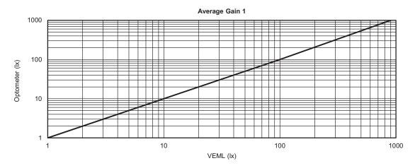
Fig. 7 - Linearity for Gain 1: Lux\_Optometer vs. Lux\_VEML6030
