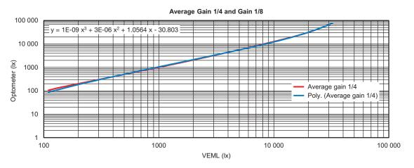
Fig. 11 - Correction Formula for Gain 1/4 and Gain 1/8 for Higher Light Levels than 100 lx
