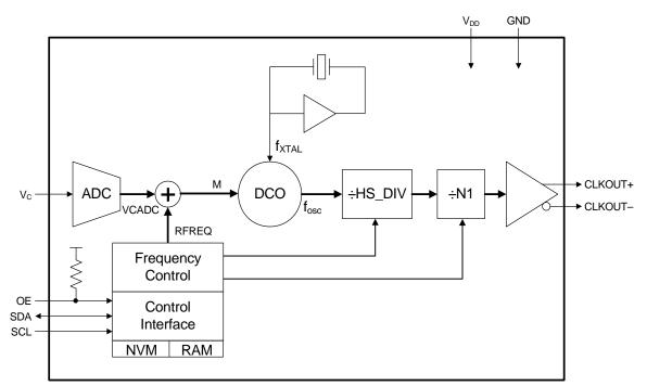
Figure 2. Si571 Detailed Block Diagram
