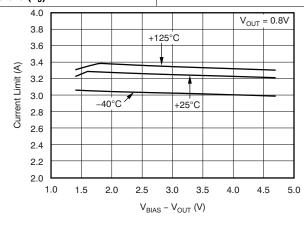
Figure 17. Current Limit vs (V<sub>BIAS</sub> - V<sub>OUT</sub>)
