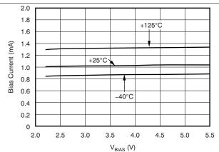
Figure 13. BIAS Pin Current vs Output Current and Temperature (T<sub>J</sub>)
