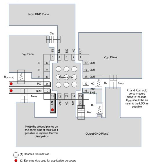
Figure 37. Layout Example (RGW Package)
