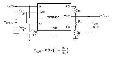
Figure 24. Typical Application Circuit for the TPS748 (Adjustable)
