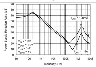
Figure 9. V<sub>BIAS</sub> PSRR vs Frequency
