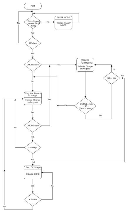
Figure 8. System-Controlled Operational Flow Chart
