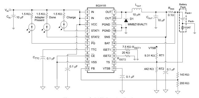
Figure 19. 1-Cell LiFePO4 Application
