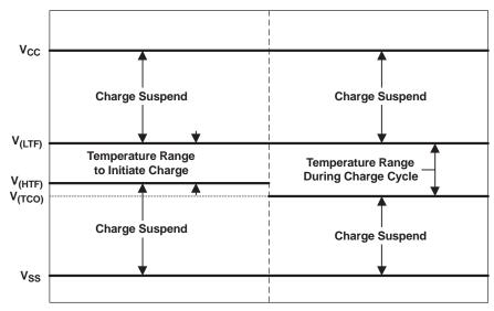
Figure 10. TS Pin Thresholds
