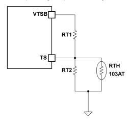
Figure 17. TS Resistor Network
