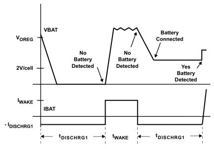
Figure 12. Battery Detect Timing Diagram
