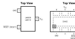
Figure 1. 3-Lead SOT-23-3 Package See Package Number DBZ () are for LM810
