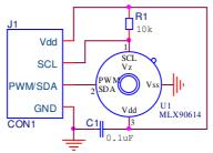
Figure 37: PWM output with SMBus available
