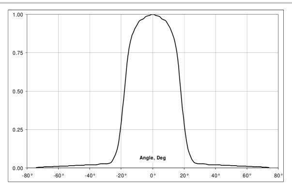
Figure 30: Typical FOV of MLX90614xCC
