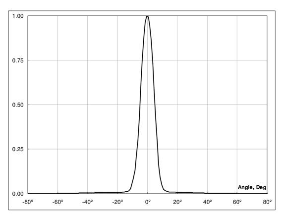
Figure 32: Typical FOV of MLX90614xCH
