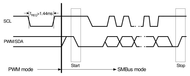
Figure 17: Switching from PWM mode to SMBus
