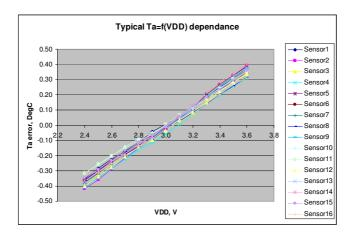
Figure 23: Typical Ta dependence from supply voltage
