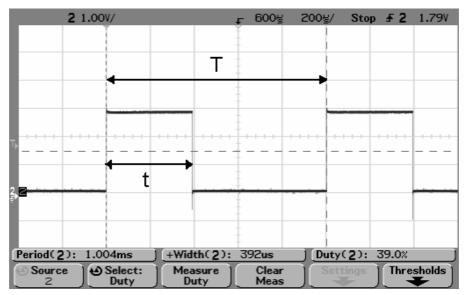
Figure 14: PWM example single mode
