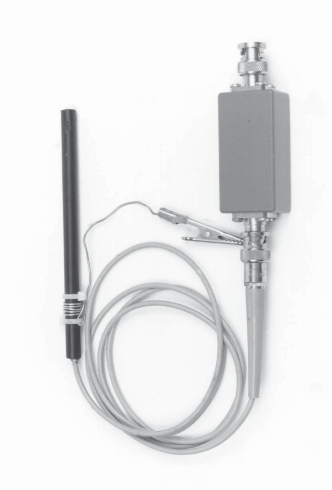
Figure C15. The Trigger Probe and Termination Box. Clip Lead Facilitates Mounting Probe, Is Electrically Neutral
