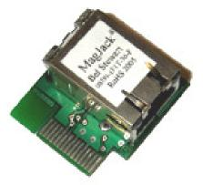
5. Connect the PICtail Daughter Board for SD & MMC Cards to the female card-edge connector J5 on the Explorer 16 board. The card-edge connector should be inserted in the center slot, with the card socket facing the microcontroller.. This will connect the PICtail Plus board to SPI2.
