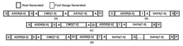
Figure 6. Supported I<sup>2</sup>C formats: (a) 1-byte write, (b) quick read, ©) 1 byte-read, and (d) incremental read (S = Start, Sr = Repeated Start, A = Acknowledge, N = No Acknowledge, and P = Stop).
