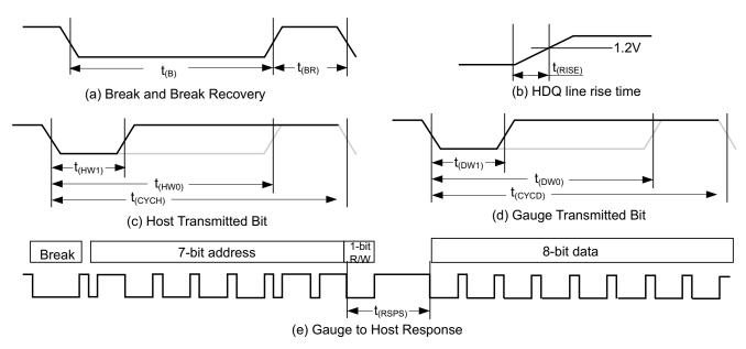
Figure 3. Timing Diagrams
