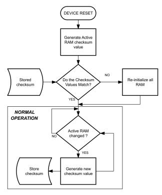
Figure 5. Partial Reset Flow Diagram
