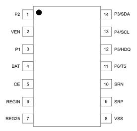
Figure 1. bq34z100 Pinout Diagram
