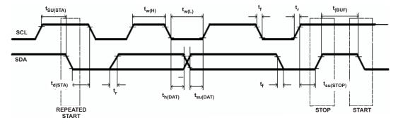
Figure 4. I<sup>2</sup>C-Compatible Interface Timing Diagrams
