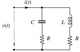
where the voltage v(t) and current i(t) are the input and output variables of the system. Determine state equations, the impulse response and the transfer function of the system. Then assume that RC = L/R is satisfied, reduce the state equations to Kalman's canonical form, and identify the uncontrollable and/or unobservable eigenvalues of the system. What are the impulse response and the transfer function of the system in this case?
