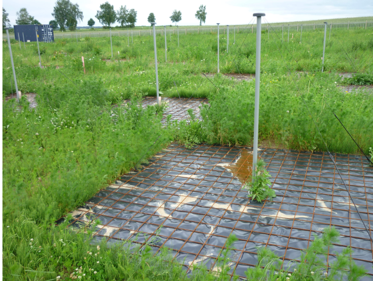
Figure 1.1. One LOFAR LBA antenna element.
