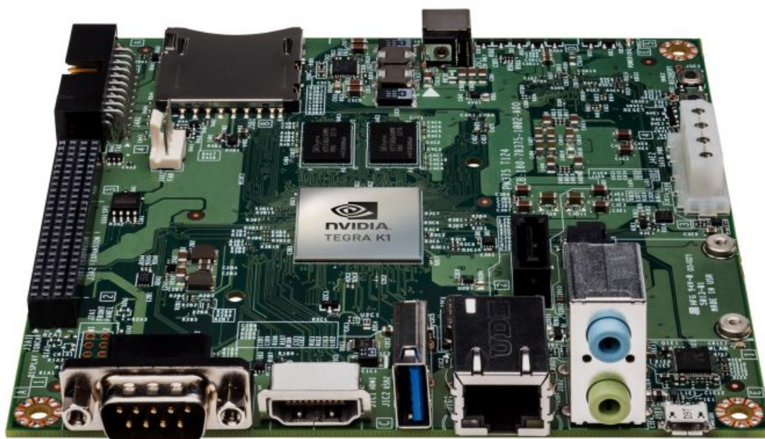
Figure 4.1. The NVIDIA Jetson TK1 Development Kit https://developer.nvidia.com/jetson-tk1 .
