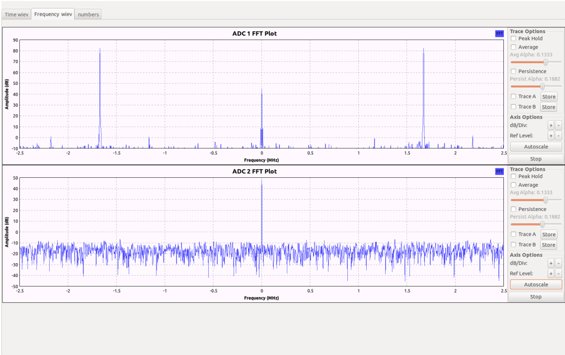
Figure 2.6. Sine signal from ADC1 module with LTC21190 and LT6600-5 devices.
