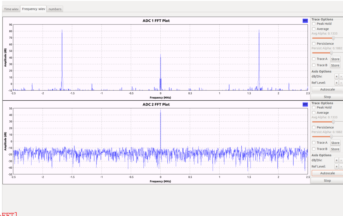
Figure 2.7. Sine signal sampled by ADC1 module with LTC2190 and LT6600-5 devices.
