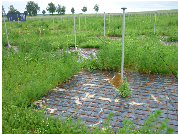
Figure 1.1. One LOFAR LBA antenna element.
