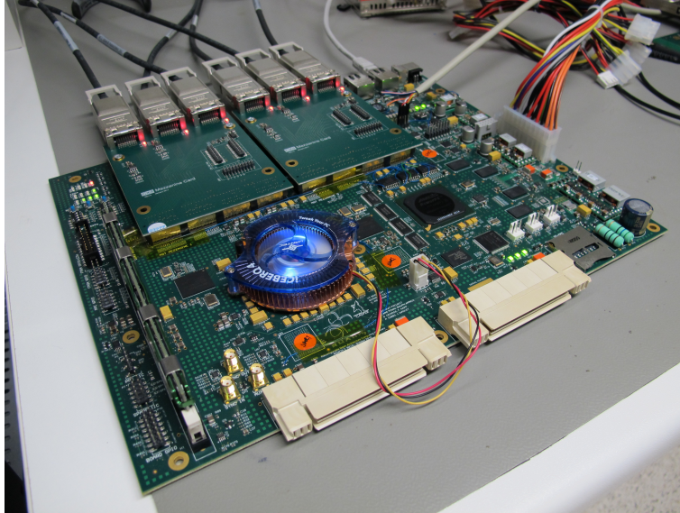
Figure 1.2. CASPER project ROACH-2 data processing board. White Z-DOK connectors for daughter ADC Boards can be easily seen in front.
