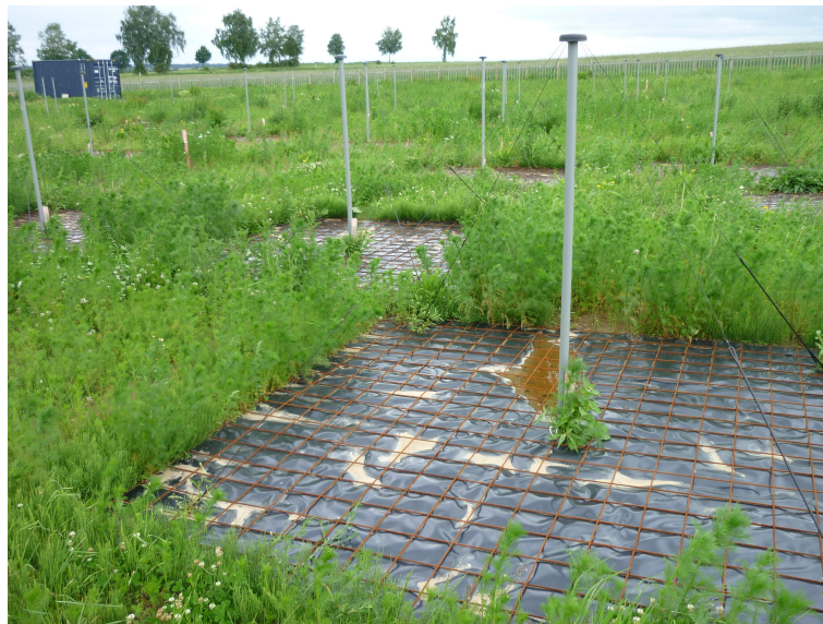
Figure 1.1. One LOFAR LBA antenna element.
