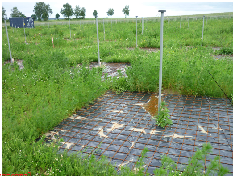
Figure 1.1. One LOFAR LBA antenna element.
