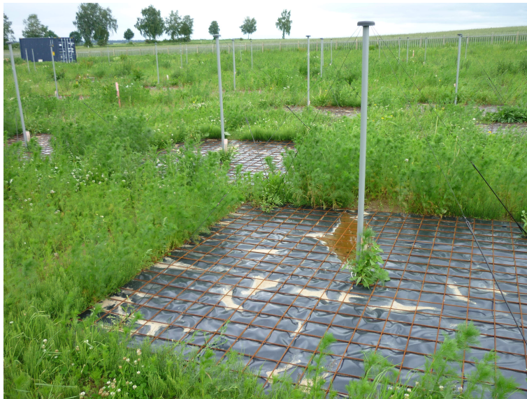
Figure 1.1. One LOFAR LBA antenna element.
