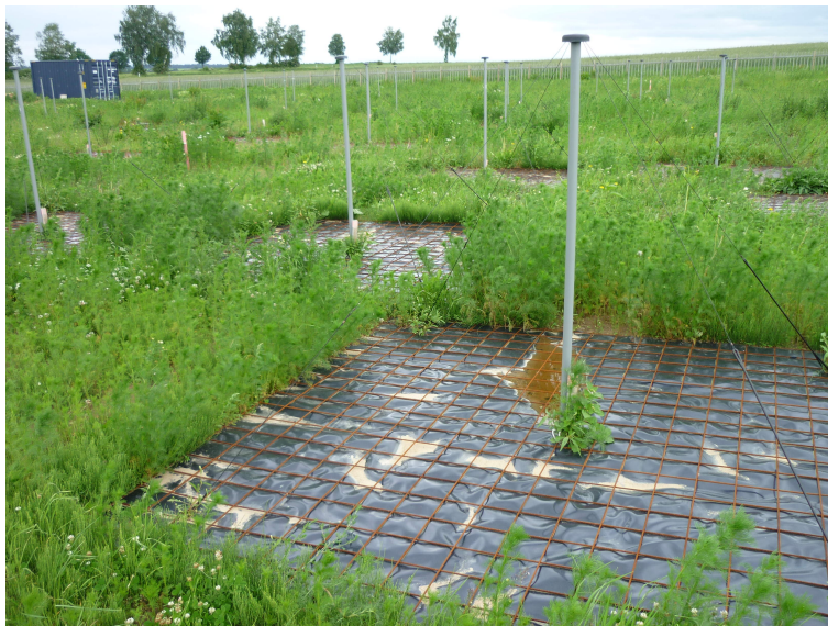
Figure 1.1. One LOFAR LBA antenna element.
