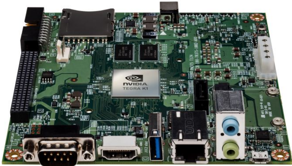
Figure 4.2. The NVIDIA Jetson TK1 Development Kit [27].
